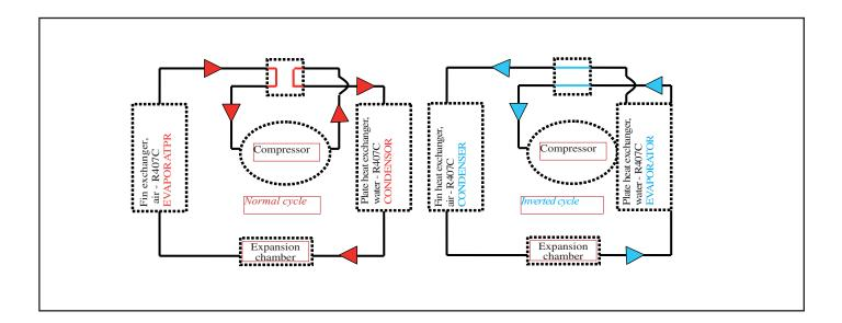
The roles of the evaporator and condenser are swapped: The fluid brings calories to the fin heat exchanger to melt the ice. The fan remains stopped while the system is defrosting. When the temperature detected by the sensor increases, defrosting is finished and the 4-way valve switches back to the normal cycle.
