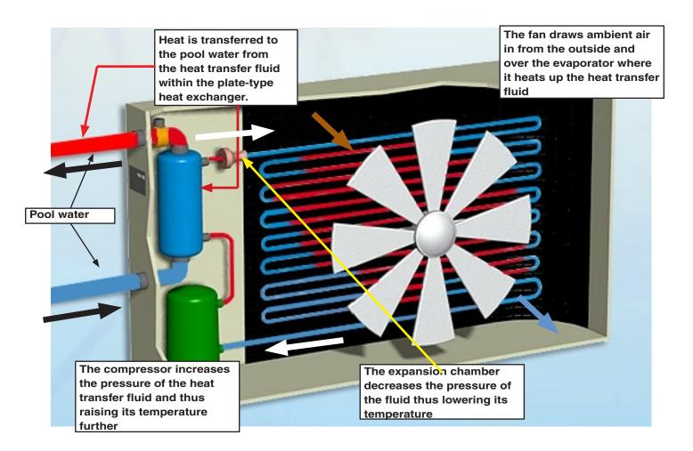
With an ambient air temperature of 15°C, CLIMEXEL heat pumps transfer 4 to 5 times more energy to the pool water than they consume (90% of this energy is consumed by the compressor): these machines have a yield (or COP - Coefficient of Performance) of between 4 and 5 (refer to the table below for the exact values for each model).
