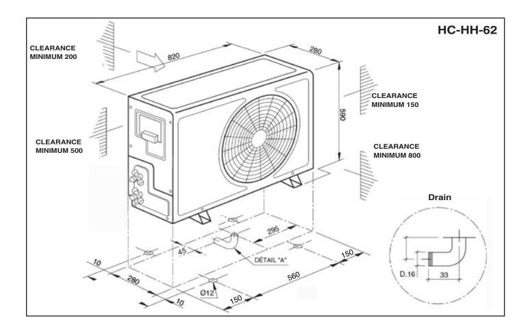
As the volume of condensates generated over time can be considerable when the ambient air is humid, water should not be allowed to accumulate around the machine: if the ground around the heat pump will not allow for the absorption or evacuation of condensates, a drainage system will be necessary.
