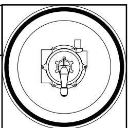
DRAIN: Water from the pump is routed directly to waste without passing through the filter.
