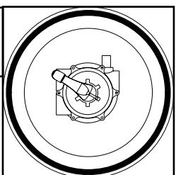
WASHING: Water from the pump passes through the filter from the bottom to the top and is then routed to waste taking with it all the impurities trapped in the filter.
