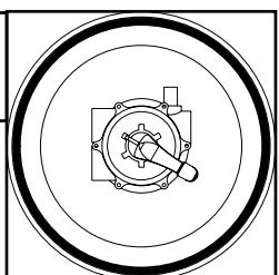
ATTENTION ! LORS DES CHANGEMENTS DE POSITION DE LA VANNE MULTIVOIES, LA POMPE DOIT TOUJOURS ÊTRE ARRÊTÉE, SANS QUOI LE FILTRE RISQUE D'ÊTRE GRAVEMENT ENDOMMAGÉ ET SA GARANTIE ANNULÉE.
