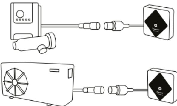
Once the iQBridge RS is connected to the device you want to control, re-connect the device (heat pump, salt water chlorinator, etc.) to the main power supply. The power ON indicateur light turns on steady green.
