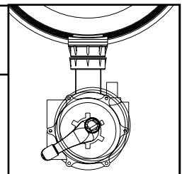
**CLOSED:** No circulation is possible. Never run the pump while the valve is in this position.
