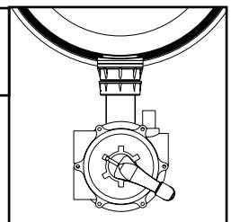
**ATTENTION ! LORS DES CHANGEMENTS DE POSITION DE LA VANNE MULTIVOIES, LA POMPE DOIT TOUJOURS ÊTRE ARRÊTÉE, SANS QUOI LE FILTRE RISQUE D'ÊTRE GRAVEMENT ENDOMMAGÉ ET SA GARANTIE ANNULÉE.**
