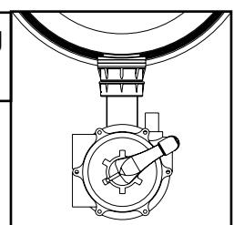
**RINSE:** Water from the pump passes through the filter from top to bottom and is then routed to waste.
