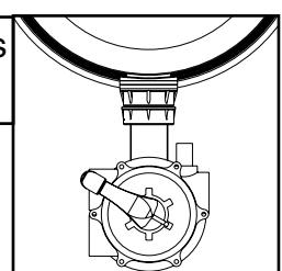
**WASHING:** Water from the pump passes through the filter from the bottom to the top and is then routed to waste taking with it all the impurities trapped in the filter.
