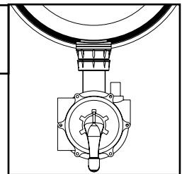
**DRAIN:** Water from the pump is routed directly to waste without passing through the filter.
