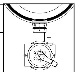
**CAUTION! NEVER CHANGE THE VALVE POSITION WHILE THE PUMP IS ON, THIS COULD CAUSE SERIOUS DAMAGE TO THE FILTER AND WILL CANCEL THE GUARANTEE.**
