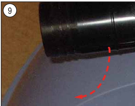
Working from underneath the cover, tighten the bronze nut by hand, then moderately using a 22 tube wrench. Take care not to damage the o-ring.
